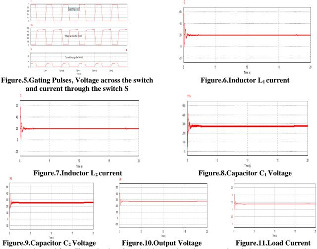
`As observed from Figure 5, when the switch is turned on, the current though the switch is zero, therefore turn on losses are reduced. The switch is turned off, when the voltage across the switch is zero. Therefore turn off losses are reduced.
