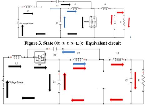
Figure.4. State  $1(t_{on} \le t \le t_{off})$ : Equivalent circuit
