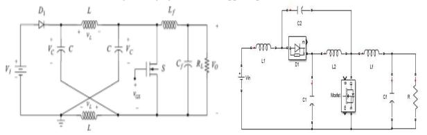
**Figure1.Voltage-fed Z-source DC-DC converter Figure.2.Voltage-fed Quasi Z-source DC-DC converter Quasi Z-Source Converter:** In Z-source converters, the input current is discontinuous and the voltage stress across the switch is more and also there is no common ground.
